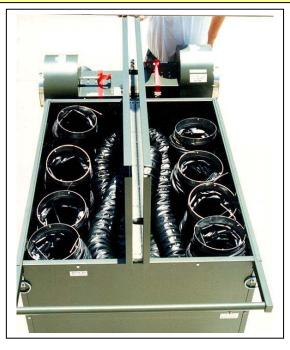
Storage of 8" (203mm) and 4" (101mm) diameter Ducting within Duct Storage compartment. NOTE: Always stand up 8"(203mm) Diameter Duct with latched stowage device to provide enough space for storage of all ducts.
