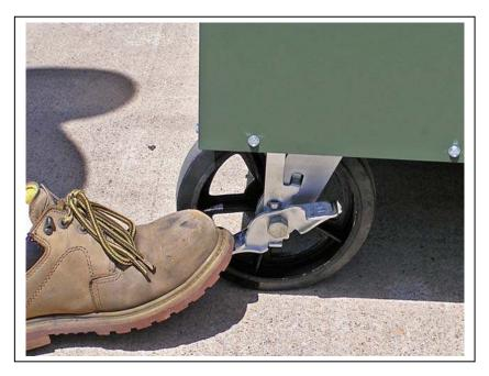
Photo showing how to manually engage and release the brake lever mounted on the storage cart swivel casters.
