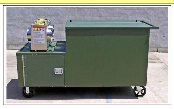
All System Components excluding the Ventilator Units are stored within the Cart. Ventilators are designed to store on top of the Cart Shelf. *NOTE: Ventilators attached Bumper Feet will fit into polarized Base Tray Mounts secured to the top of the Storage Cart Shelf.*
