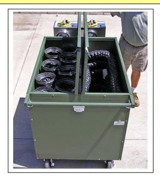
Storage of 8" (203mm) and 4" (101mm) diameter Ducting within Duct Storage compartment. *NOTE: Always stand up 8"(203mm) Diameter Duct with latched stowage device to provide enough space for storage of all ducts.*
